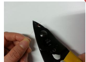
2b/ If for 250 or 900µm cable, strip off around 35mm coating, then jump to point 6.
