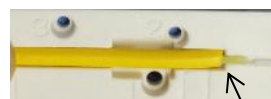
a/ For 2mm or 3mm cable, set the cable edge at above shown point.
