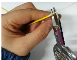
3/ Cut Kevlar to the length of 4mm.
