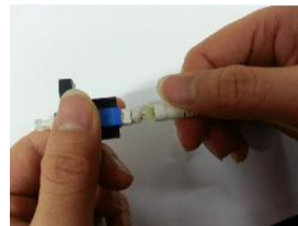
3/ Unscrew the boot and remove cable gently.
