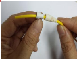
1a/ For 2mm or 3mm cable, slide the boot and lock nut onto cable.
