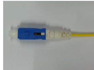
6/ Release wedge clip and termination is done.
