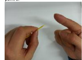
6/ Check the fiber integrity by bending the stripped end slightly at 60° in multi-directions.
