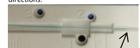
b/ For 250 or 900µm cable, set the fiber edge at above shown point.
